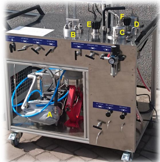
CO2 pump (A); reactor top flange (B); Separator vessels (C,D); manual pressure controls (reactor, E, separator (F)
